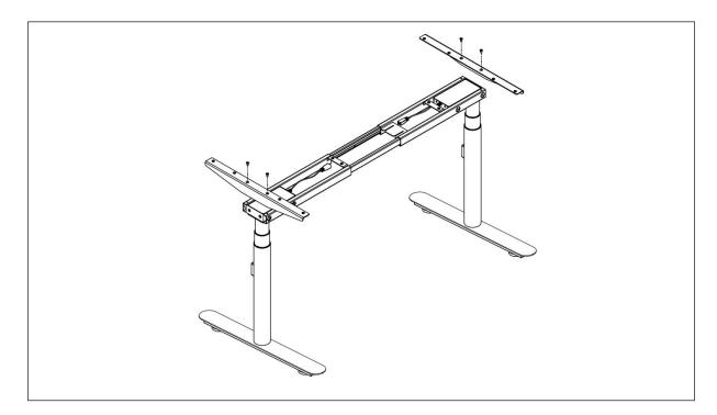
Mount the tabletop and fix it with 14 pcs screws ST4x20; Tighten the screws like D display to fix the top frame.Fix the centre bracket with 2 pcs screws M6x10
