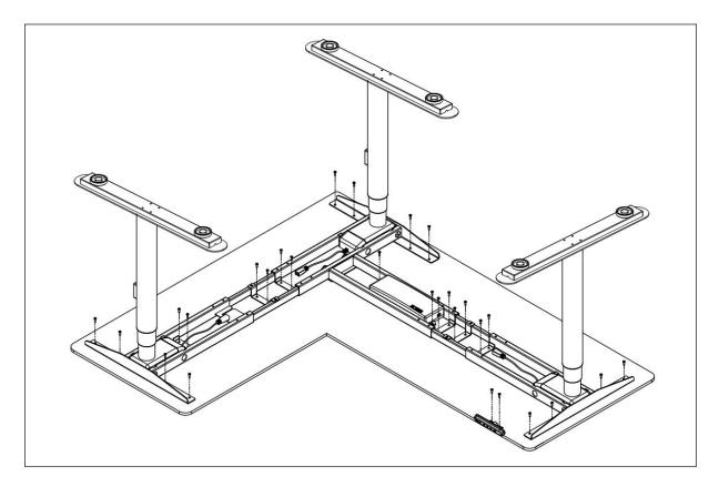
Mount the control box to the frame, fix the handset with 2pcs screws ST4x20. Connect the cables and zipped it with cable tie.
