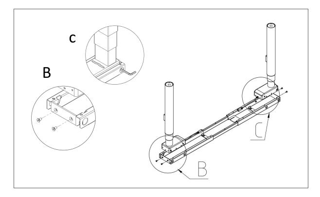
Install the two table feet with Screws 8 pcs M6x16, Install the 4 pcs leveling pads
