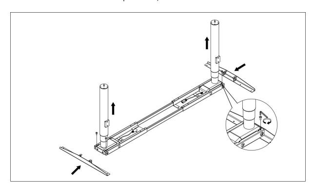
**Step 4** Install the leveling pads
