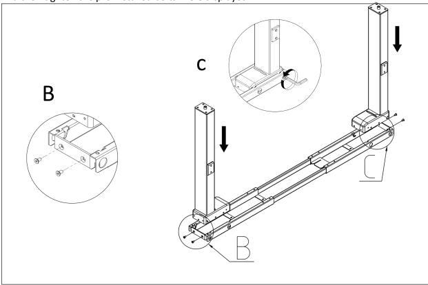
**Step 3**Install the side brackets with Screws 8 pcs M6x16,
