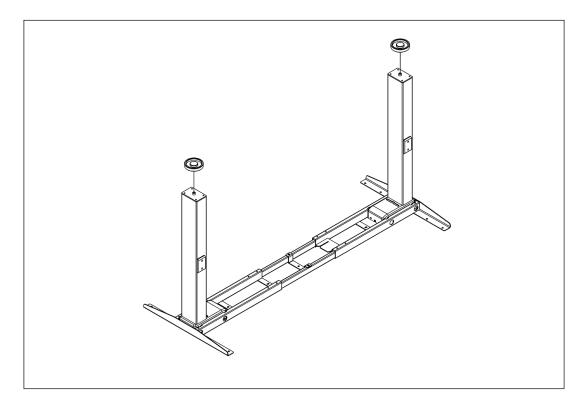
**Step 5**Install the connected pipe with 8 pcs screws M8x10
