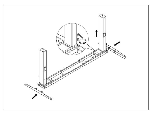
**Step 4** Install the leveling pads
