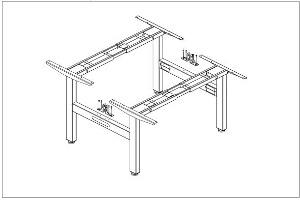
**Step 7**Fix the table top with 26pcs screws ST4x20 ,Install the centre bracket with 4 pcs screws M6x10
