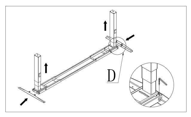
**Step 4** Install the leveling pads
