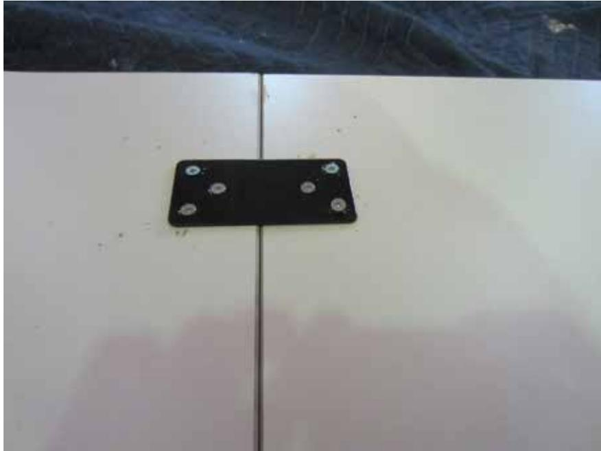
**4. Place the legs upside down on the desk top as below. The leg with the motor attached will go the side with the additional top piece. The middle leg will be parallel to the leg with the motor. The final leg will be 90 degrees to the other legs.**
