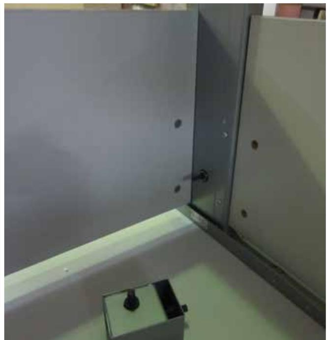
**8. You can now position the legs on the table (around 95mm from the edge of the top). Make sure to leave enough of the table hole uncovered to allow any plugs/cords to fit through.**
