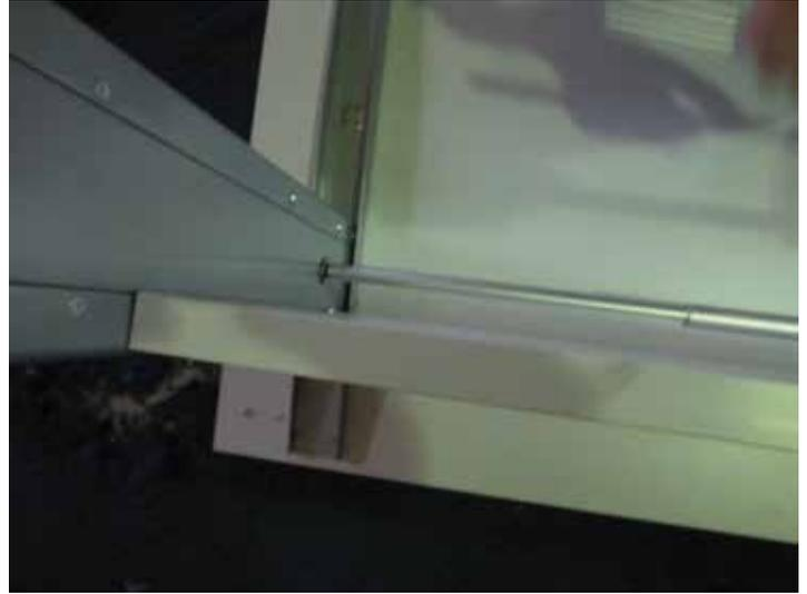
**15. Use the provided alan key to screw the stoppers into place which will keep the rods in the extended position.**
