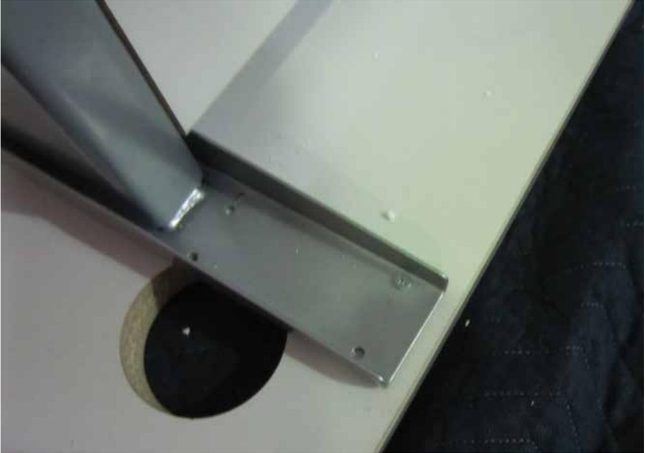
**11. To position the transmission on the middle leg you will need to remove the lower bolt. Use an allen key to unscrew the bolt.**
