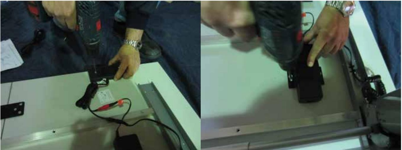
**20. Flip over the desk so that it is no positioned on its feet. Attached the plug to the power supply and your desk is now ready to use.**
