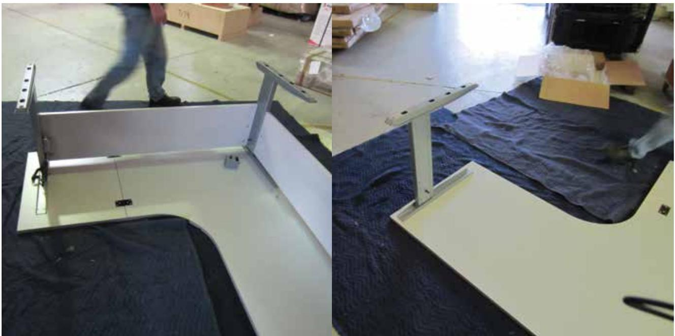
5. The length of the modesty panels will determine where the desk legs can be positioned. The shorter modesty panel will go between the leg positioned at 90 degrees and the middle leg. The longer modesty panel will go between the middle leg and the motor leg.
