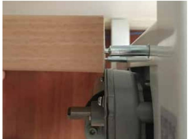
7. Place the cam locks in the holes and tighten to secure the modesty panel to the legs.
