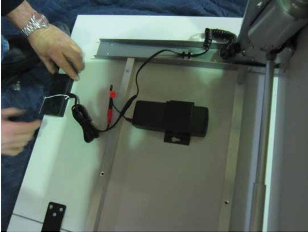
**19. Make sure the height adjustment switch is lined up with the edge of the desk. Screw the switch and power supply into position.**
