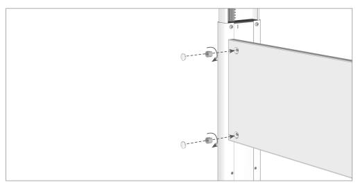
**STEP 2:** Slide modesty panel into position on each leg, tighten cam to lock in place. Use a soft headed hammer as necessary to fit the plastic cover caps to each cam.
