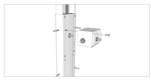
STEP 1: Secure the gear transfer box to the centre leg. Remove screw from leg first, slide on transfer box, then securely tighten screw back in place. Follow steps 1 to 7 of the desking assembly guide to assist in workstation assembly.
