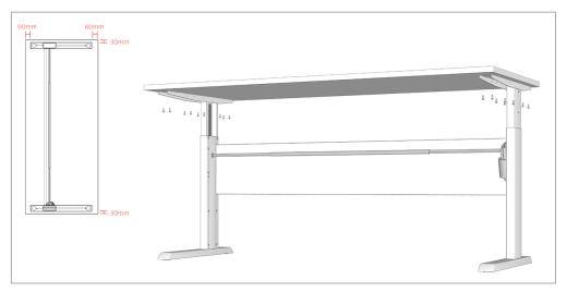
**STEP 5:** Secure the worksurface to each leg using the provided screws.
