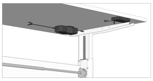
**STEP 6:** Secure the power supply and controls in the locations pictured below. Ensure the controls are located near the front edge of the worksurface.
