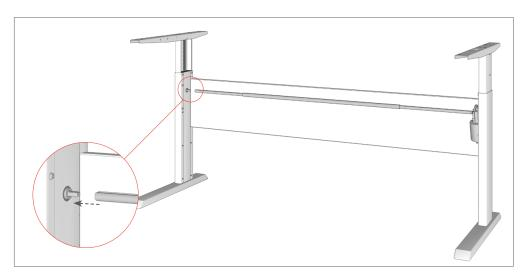
**STEP 3:** Slide the gear rail onto the opposite leg to the motor, then fully extend the rail until it meets the drive shaft on the motor.
