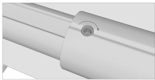
**STEP 4:** Once the gear rail is fully extended, tighten the 2 small grub screws on the rail to secure the rails length.
