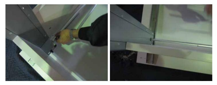
15. Use the provided alan key to screw the stoppers into place which will keep the rods in the extended position.
