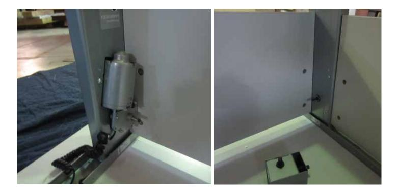
8. You can now position the legs on the table (around 95mm from the edge of the top). Make sure to leave enough of the table hole uncovered to allow any plugs/cords to fit through.
