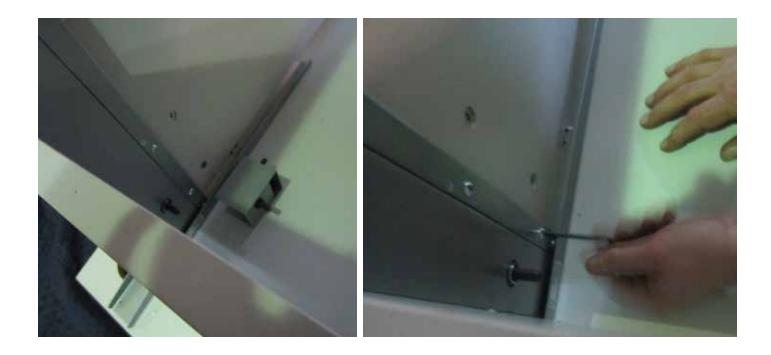
12. Place the transmission in place as below and use the alan key to place the bolt back in its original position.
