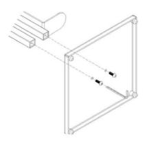
Slide the **Bottle Holder** onto the **Frame** to the desired height as shown below.
