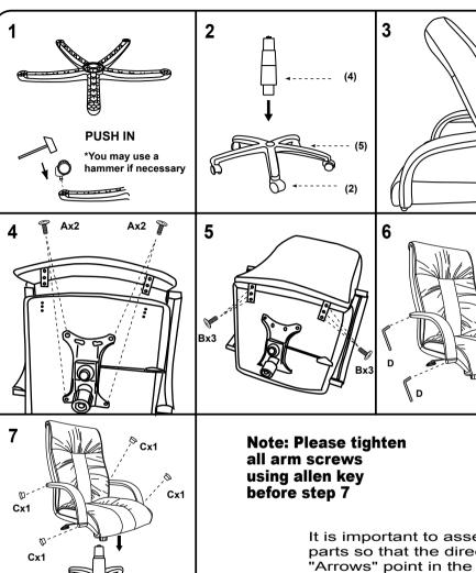
It is important to assemble all parts so that the directional "Arrows" point in the same direction. Make certain that all screws are FULLY tightened before using the chair. Each month, check all screws and tighten any that may have loosened.
