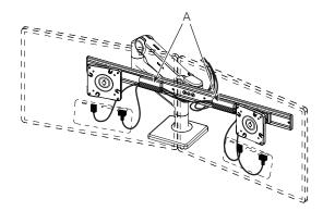
2. Route power and monitor cables through the flexible cable clips on the M8.1's upper link (B).
