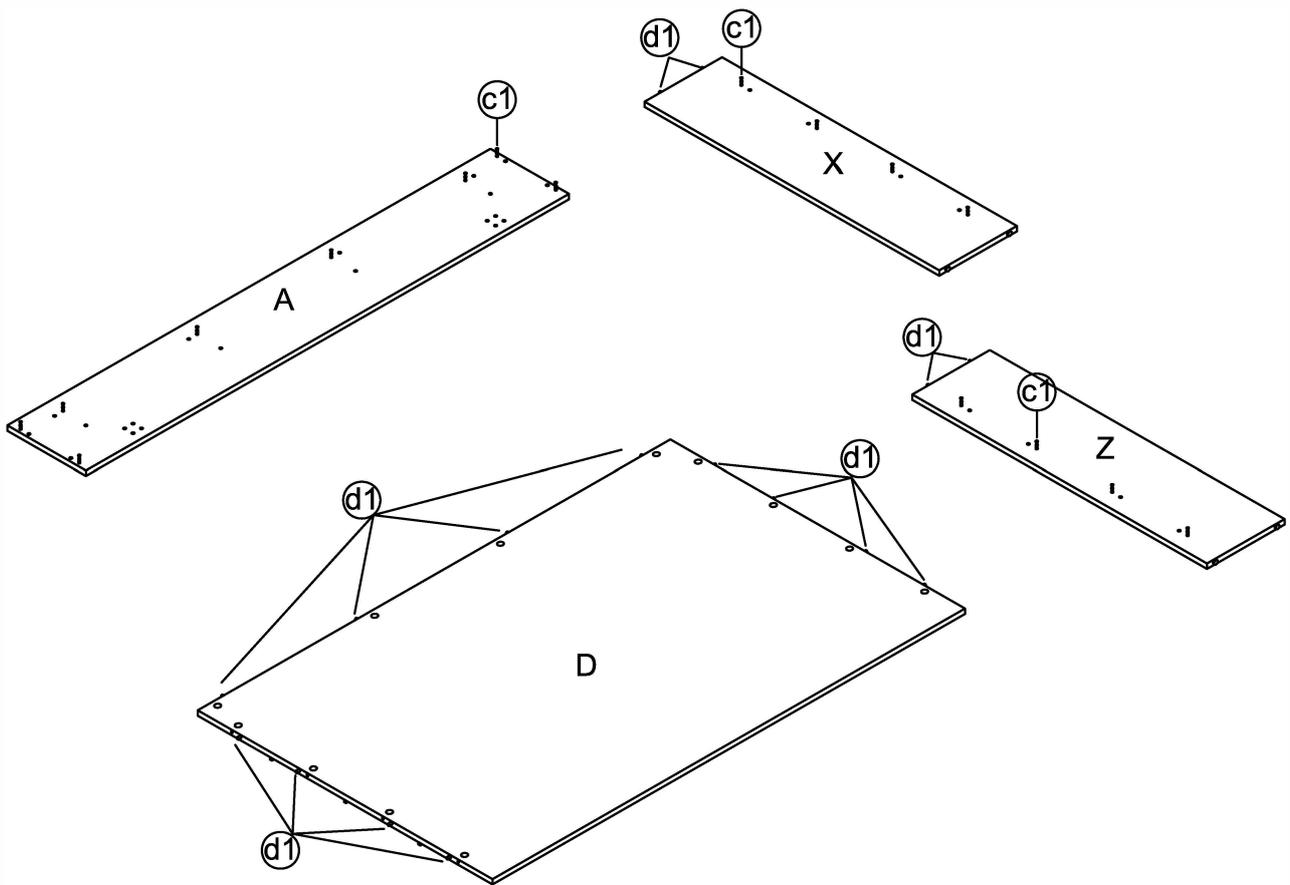
**Preparation for Top panel A, Back panel D, Left side panel X, Right side panel Z .**
