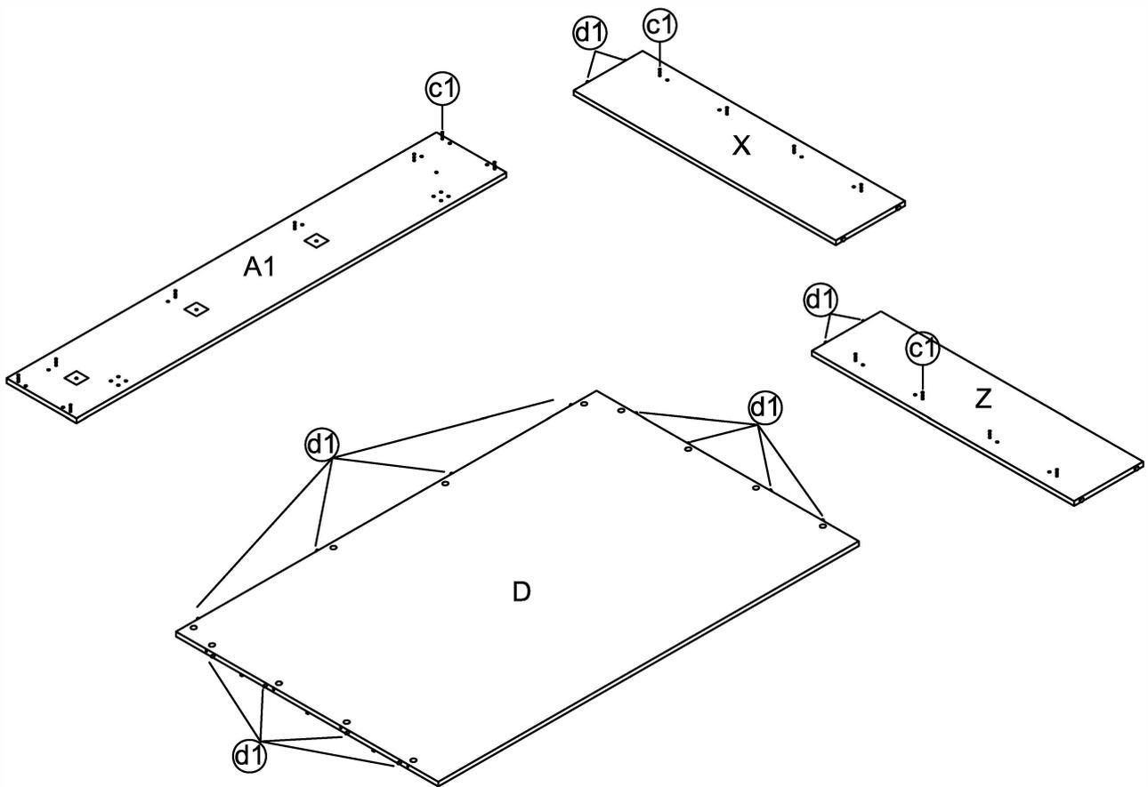
**Preparation for Top panel A1, Back panel D, Left side panel X, Right side panel Z .**
